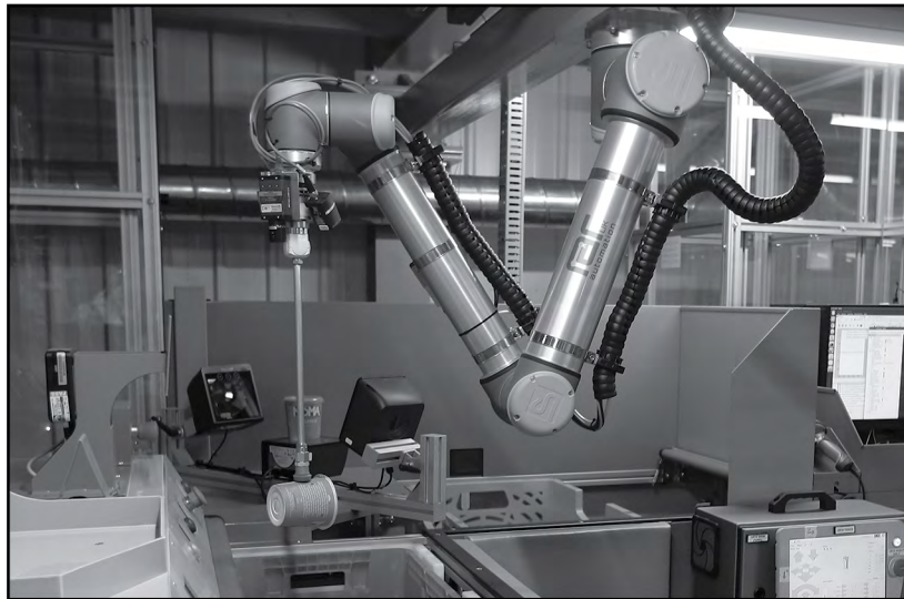
Ocado's experimental industrial robot arm, designed to take over the work currently done by human "pickers."
